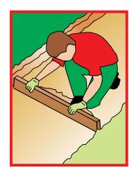
Compact the soil with a garden roller and then spread the sand with a rake and level it by scraping and tamping with a length of timber. To support heavier loads, or if the soil is composed of clay or peat, lay a subbase of firmly compacted hardcore (broken bricks or crushed stone) to a depth of 75 to 100mm before spreading the sand to level the surface. If you plan to park vehicles on the paving, increase the depth of hardcore to 150mm.
