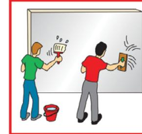
5. Wet the leveled plaster with water (flicked off a brush), then use a wood float to smooth the surface.
