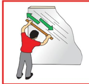
4. Once the plaster starts to stiffen, level the surface by pulling a wooden straight edge tool over the plaster with a swaying motion.
