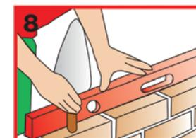
Hold the spirit level along the outer edge of the bricks to check that they are in line. To move a brick sideways without knocking it off its mortar bed, tap the upper edge with the trowel at about 45°.
