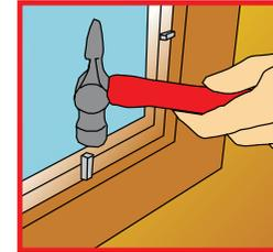
Working from the outside, put the pane of glass in the bedding putty and press it gently into place. Do not press the centre of the pane as this may cause it to crack. Tap in panel pins until they are flush with the glass, using a hammer. The hammer head should slide gently against the glass to secure the sprigs. (Do not aim blows as if you were knocking in a nail).
