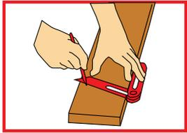
When using the sliding bevel it is essential to ensure that the stock of the tool is held firmly against the edge throughout the marking procedure.
